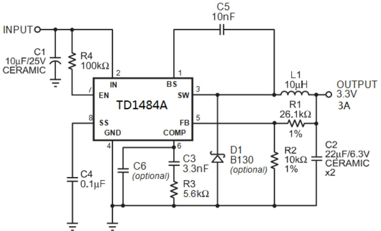
Fig17. TD1484A with 3.3V Output, 22µF/6.3V Ceramic Output Capacitor
