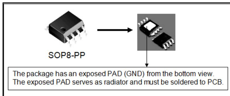
Figure 1. Package Types of TD1484A
