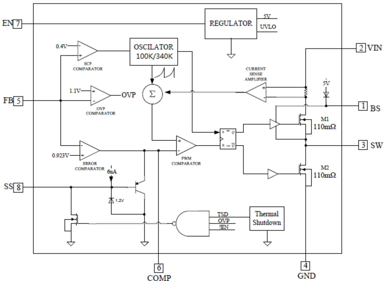
Figure 3 Function Block Diagram of TD1484A
