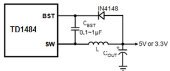
Figure18.Add Optional External Bootstrap Diode to Enhance Efficiency
