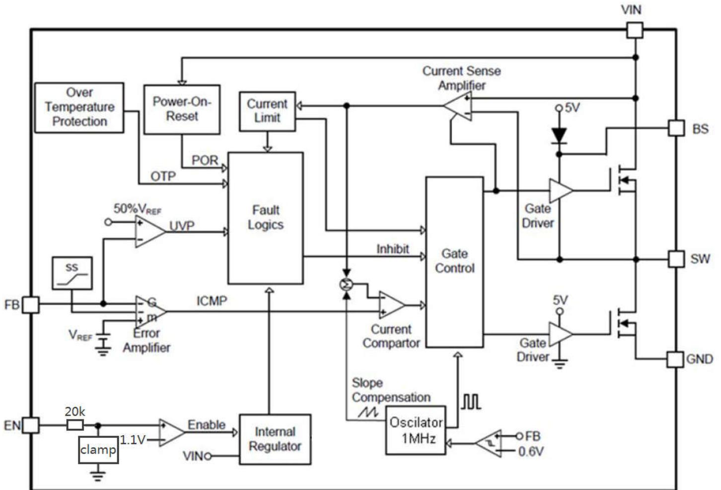
Figure1 Function Block Diagram of TD1469
