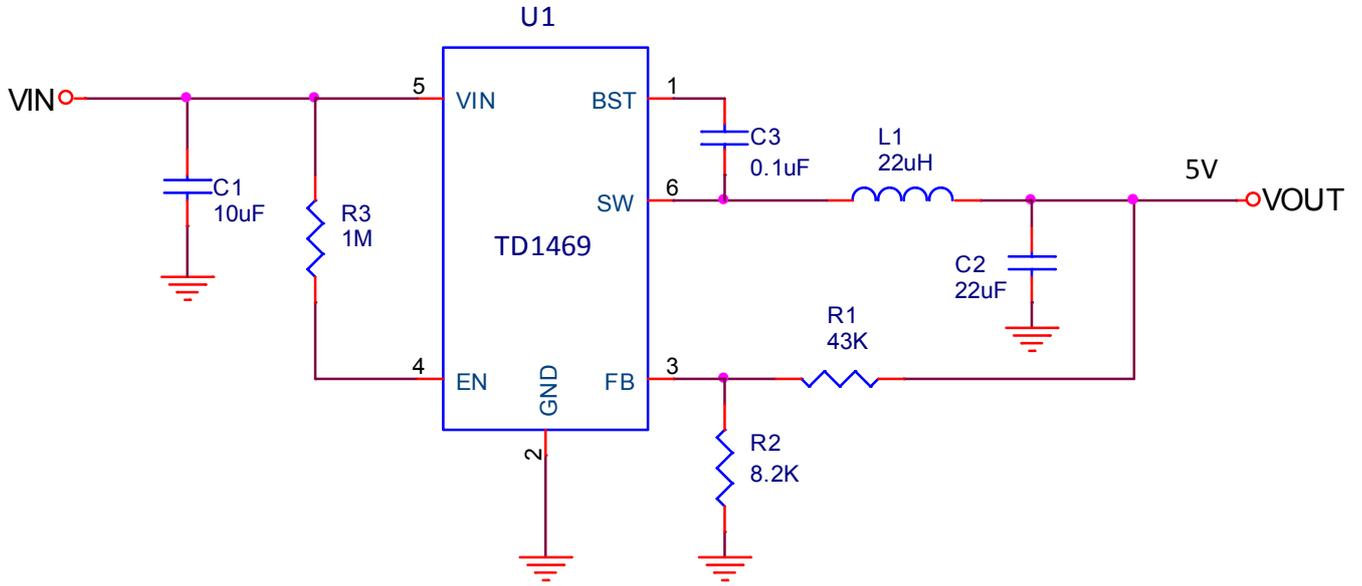
$$V_{OUT} = V_{REF} \left( 1 + \frac{R1}{R2} \right)$$
