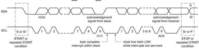
Figure 7 Data transfer on the I2C bus
