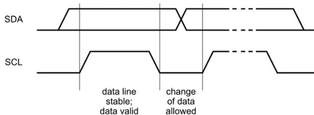
Figure 5 Bit transfer on the I2C bus
