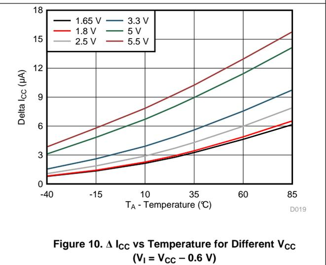
Figure 10. Δ I<sub>CC</sub> vs Temperature for Different V<sub>CC</sub> (V<sub>1</sub> = V<sub>CC</sub> - 0.6 V)
