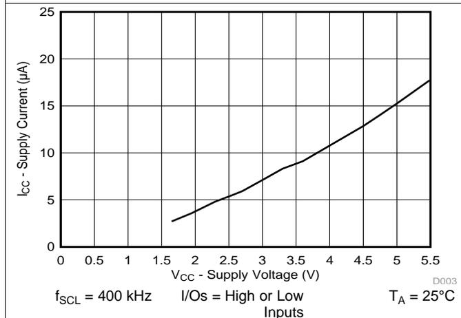
Figure 3. Supply Current (I<sub>CC</sub>, Operating Mode) vs Supply Voltage (V<sub>CC</sub>)
