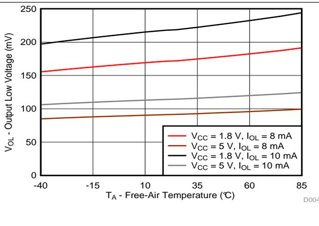
Figure 4. Output Low Voltage (V<sub>OL</sub>) vs Temperature (T<sub>A</sub>) for P-Port I/Os
