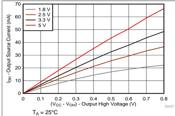
Figure 7. Source Current (I<sub>OH</sub>) vs Output High Voltage (V<sub>OH</sub>) for P-Ports at Four Supply Voltages
