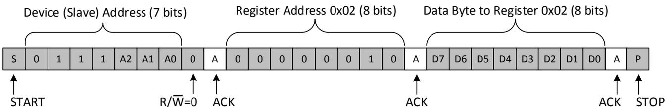
Figure 22. Write to the Polarity Inversion Register
