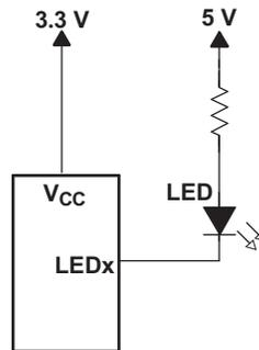
Figure 28. Device Supplied by a Lower Voltage
