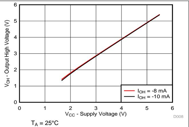
Figure 8. Output High Voltage (V<sub>OH</sub>) vs Supply Voltage (V<sub>CC</sub>) for P-Ports
