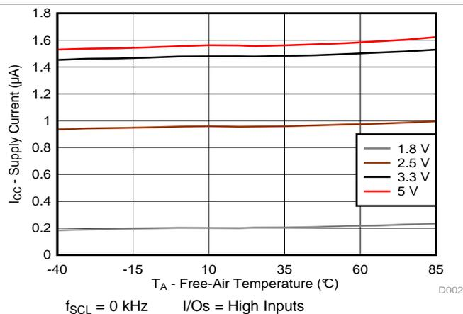
Figure 2. Supply Current (I<sub>CC</sub>, Standby Mode) vs Temperature (T<sub>A</sub>) at Four Supply Voltages
