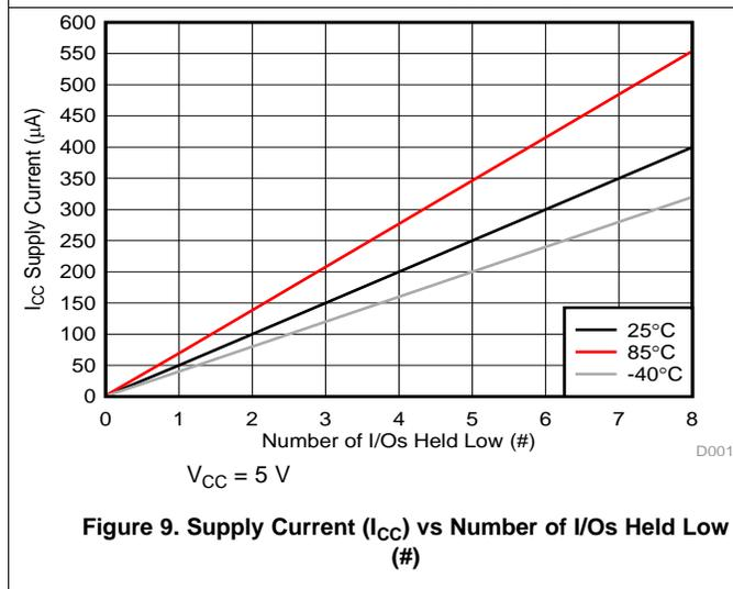
Figure 9. Supply Current (I<sub>CC</sub>) vs Number of I/Os Held Low (#)
