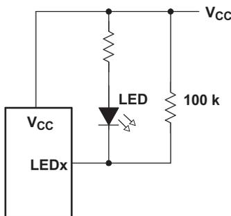
Figure 27. High-Value Resistor in Parallel With LED
