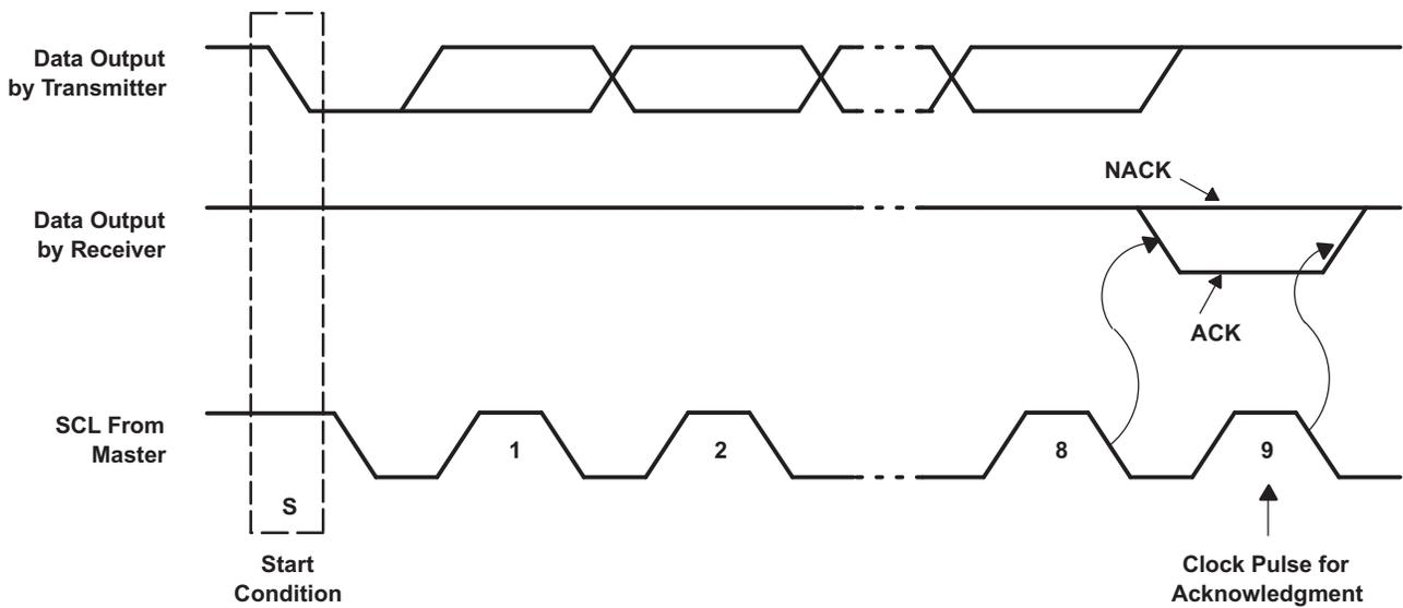
Figure 18. Acknowledgment on I<sup>2</sup>C Bus
