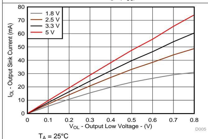
Figure 5. Sink Current (I<sub>OL</sub>) vs Output Low Voltage (V<sub>OL</sub>) for P-Ports at Four Supply Voltages
