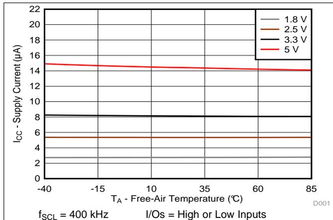
Figure 1. Supply Current (I<sub>CC</sub>, Operating Mode) vs Temperature (T<sub>A</sub>) at Four Supply Voltages
