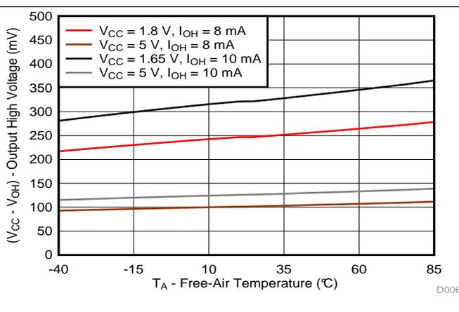
Figure 6. Output High Voltage (V<sub>CC</sub> - V<sub>OH</sub>) vs Temperature (T<sub>A</sub>) for P-Ports
